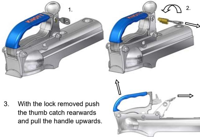
3. With the lock removed push the thumb catch rearwards and pull the handle upwards.
