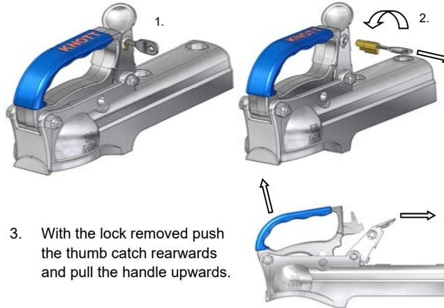
3. With the lock removed push the thumb catch rearwards and pull the handle upwards.
