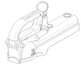
Ideally the Drawtube diameter should be between 32mm & 62mm
