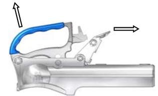
4. Lower the coupling head onto the towball.
