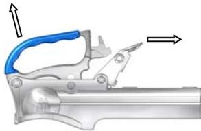
4. Lower the coupling head onto the towball.
