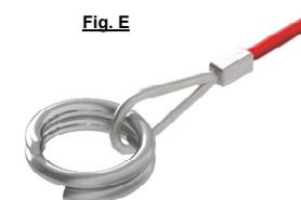
1. Where a coil fitting is used on the handbrake, use pliers and screwdriver to prise the coils of the retention ring apart and remove the ring from the handbrake lever. See Fig. E.
