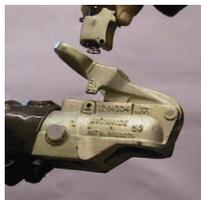
3. If the housing is not currently fitted with a lock, remove the spring and re-use. Remove the washers and the plastic blanking plug and discard.
