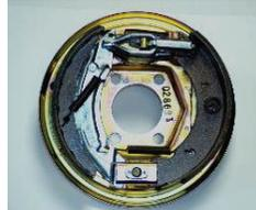
9. With care and using a suitable lever, lift sliding shoe carrier away from expander. Extract expander and retain. **NOTE.** Auto adjust assemblies are supplied complete.
