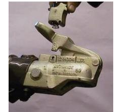
2. Using a punch drift the pin out allowing the lock housing to lift off. See Fig. F.
