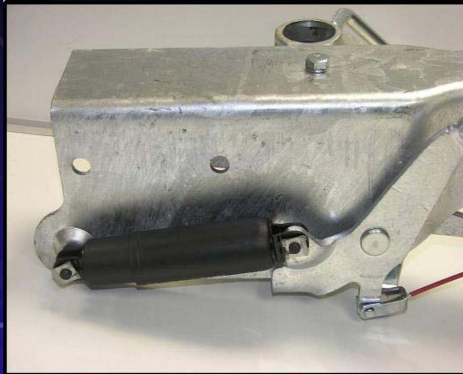
Another leading edge technology feature. The oil damping to the spring in the energy store allows gentle and progressive application of the handbrake once the handbrake has passed “over centre”. No more sudden surprises or even injuries.
