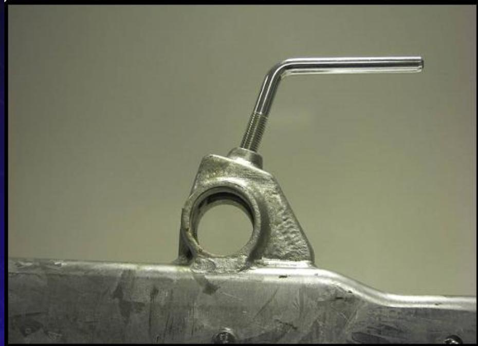
The **locking handle** is wound into the jockey bracket and the pressure pad slots over the end of the handle. The handle then withdraws the pad securely into the housing casting where it is retained, making it impossible for either the pad or the handle to be lost. The handle is M16 so extremely robust.
