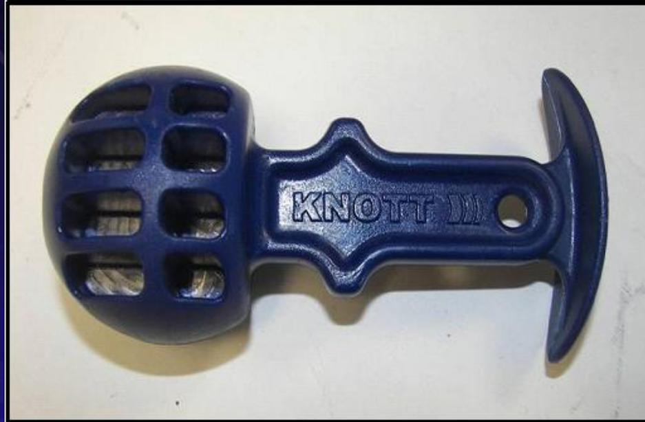
Knott introduces a new safety and security feature with their **blue ball**. The blue ball is fitted into the coupling head and then locked once the trailer is uncoupled from the towing vehicle. This allows the primary locking and security feature to be applied on the coupling head but more crucially prevents any unauthorised person from connecting the head to an undersized ball or other spurious connection.
