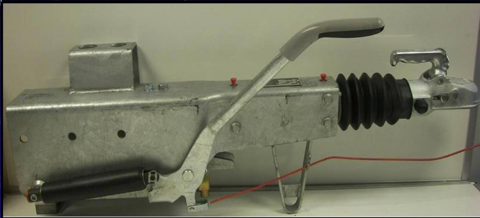
The **KRV35** completes our range of pressed steel square tube couplings taking the MGW up to 3500kg. This very robust coupling fits on to 120mm square tube and features many of the benefits seen throughout our coupling range. These include the oil damped energy store, integral skid, our bespoke overrun damper, easy-fit breakaway cable and comprehensive range of towing heads and eyes etc. This coupling is ideal for heavier drawbar applications such as boat trailers.
