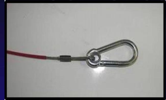
The **breakaway cable** is one of the most important mandatory components on the trailer. It needs regular checking and, if damaged, replacing. Knott has designed a simple method of replacement with a clevis and pin instead of a difficult burst ring. The carabiner style front fitting allows simple attachment to a fixed point on the towing vehicle.
