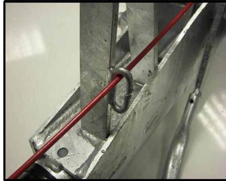
**All Knott couplings can be supplied with a cable guide for the breakaway cable. This is either a simple pressing that can be fitted under the nut of the coupling head bolt, or as a loop on the safety skid (on the square tube couplings). This guide ensures that, in the unlikely event of the trailer detaching from the towing vehicle, the breakaway cable will pull in the forward direction and apply the handbrake lever correctly.**
