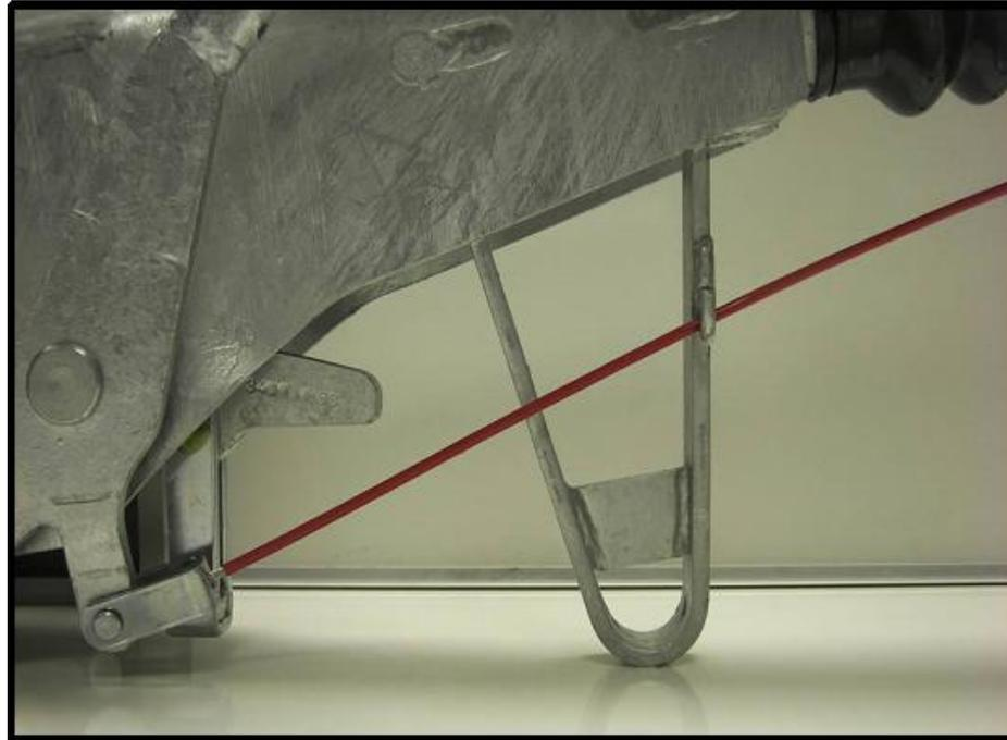
**Another longstanding feature on all square tube couplings since 1993, the skid is an integral feature of the square tube housing and protects the overrun lever and handbrake lever from damage from sleeping policemen and other objects under the trailer. This feature is mandatory in many European countries.**
