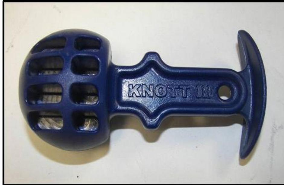
**Knott introduces a new safety and security feature with their blue ball. The blue ball is fitted into the coupling head and then locked once the trailer is uncoupled from the towing vehicle. This allows the primary locking and security feature to be applied on the coupling head but more crucially prevents any unauthorised person from connecting the head to an undersized ball or other spurious connection.**
