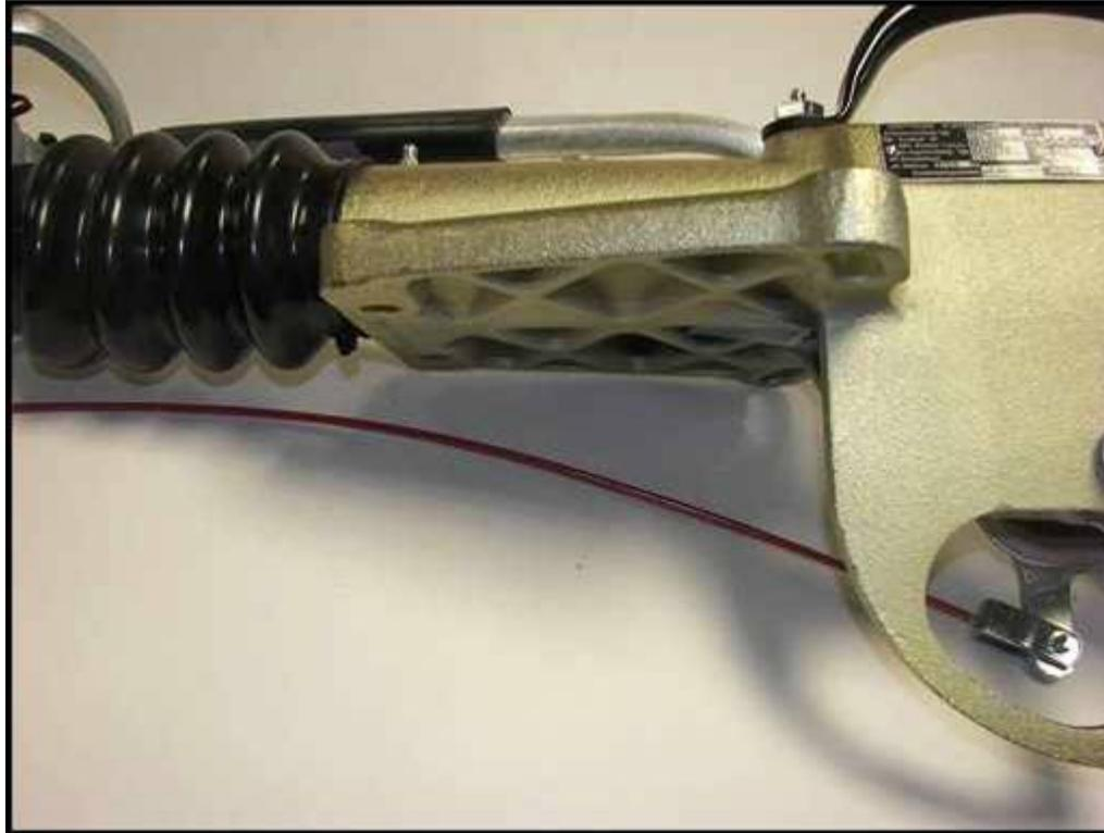
**The Knott cast housing is a typically thicker cast section with additional strengthening through a lattice form to the base and thus extremely robust. Coupled with this, the integral machined cast bearing spread is longer and thus more supportive leading to less wear and longer life.**
