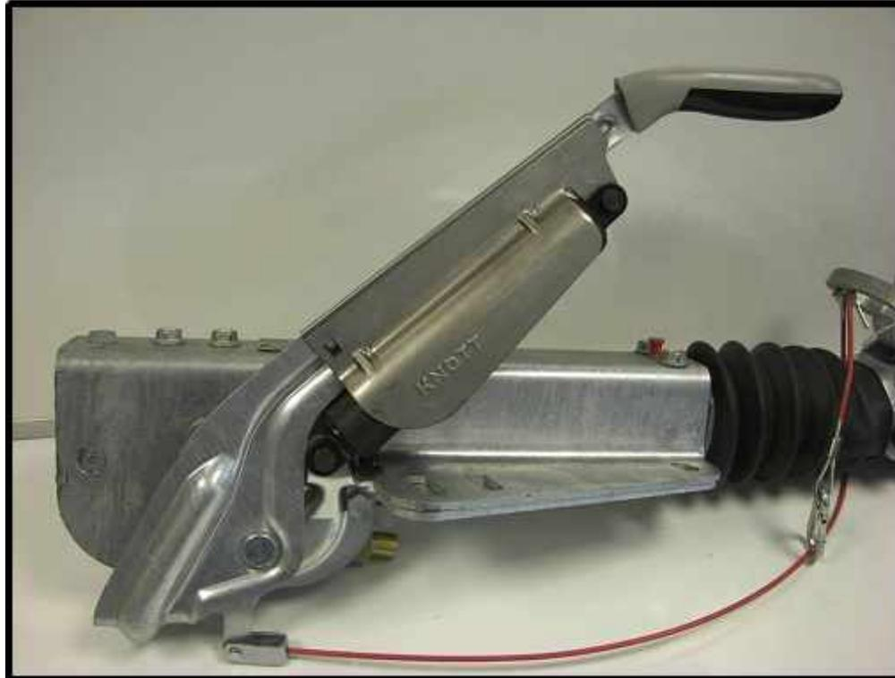
**This variation of our oil damped handbrake lever offers the opportunity to reduce the overall length of the coupling, removing the energy store support bracket and mounting the damper within the handbrake lever. This can be beneficial when there is a need to mount items on the “A” frame which might otherwise conflict with the energy store mounting bracket.**
