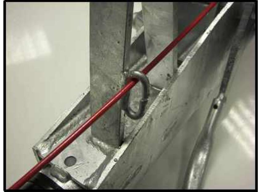
**All Knott couplings can be supplied with a cable guide for the breakaway cable. This is either a simple pressing that can be fitted under the nut of the coupling head bolt, or as a loop on the safety skid (on the square tube couplings). This guide ensures that, in the unlikely event of the trailer detaching from the towing vehicle, the breakaway cable will pull in the forward direction and apply the handbrake lever correctly.**
