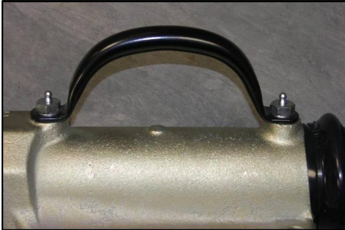
**The grab handle has been a standard feature on Knott cast couplings since 1993. This enables easy manoeuvring of the trailer without handling the coupling head, towing eye or handbrake lever which often leads to damage or dirty hands.**
