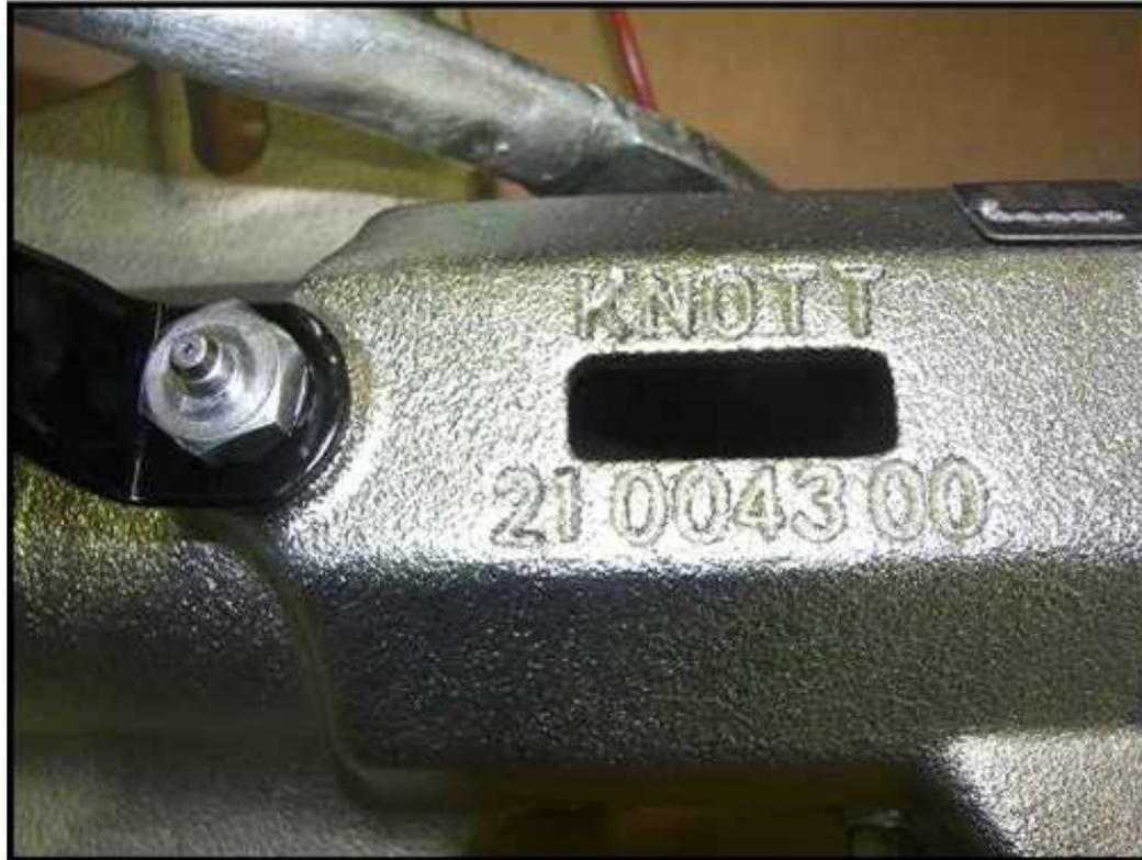
**Whilst Knott can offer a manual reverse lock on the heavier cast couplings, the compatibility of the Knott coupling with its own brake is clearly unrivalled and thus, if the brakes are reasonably and regularly serviced, such a device is rarely if ever needed.**
