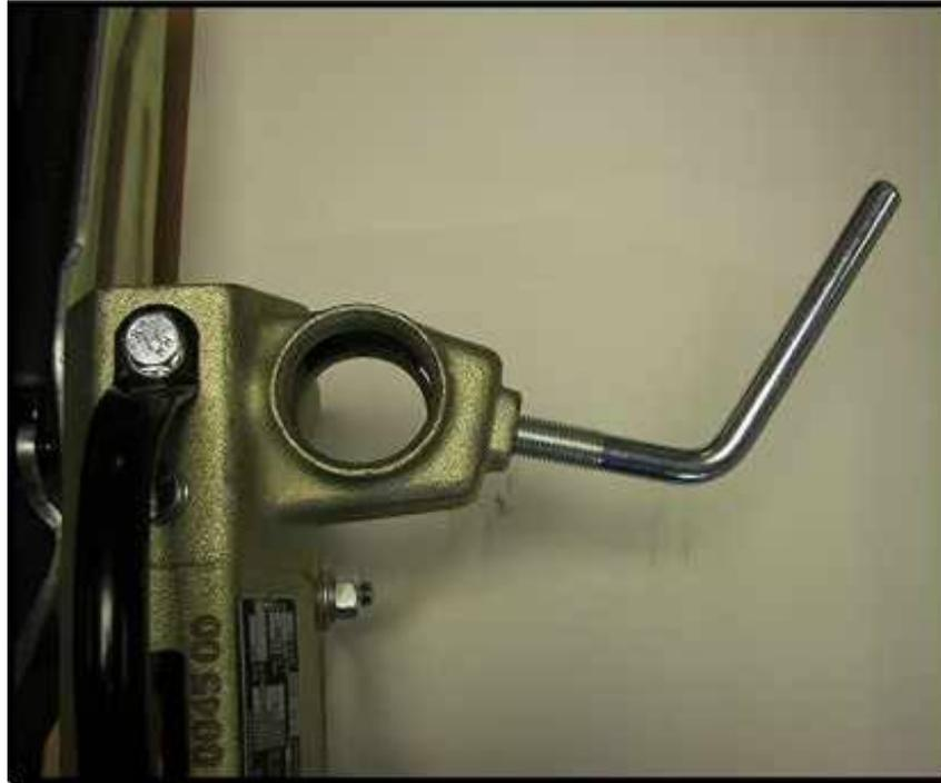
**All Knott couplings have the option of a 48mm jockey wheel facility (standard on ALL cast couplings) so that a more robust 48mm jockey wheel or even the serrated jockey can be used on any capacity of trailer. The jockey clamp is also slightly rearward of the rear mounting holes allowing easier stowing of the tyre inside of the “A” frame.**
