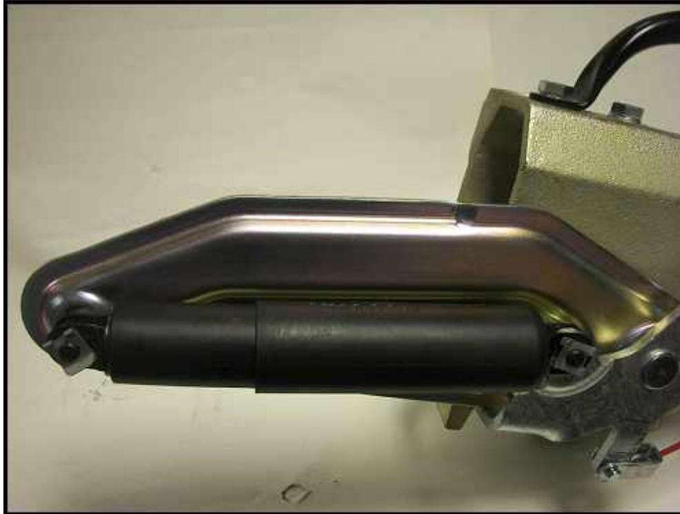
**Another leading edge technology feature. The oil damping to the spring in the energy store allows gentle and progressive application of the handbrake once the handbrake has passed “over centre”. No more sudden surprises or even injuries.**
