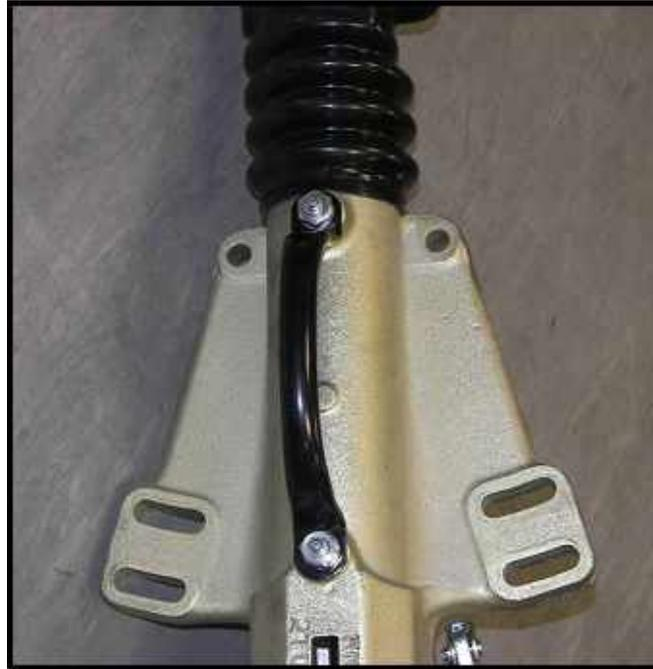
**With 4 rear holes on the KFG35, Knott offers a more secure coupling mounting by using the two front holes and the 2 rearmost holes or even all 6! The slots on all four rear holes also allows for variations in “A” frame angles, allowing the “A” frame to be narrow or wide dependent on the design requirement.**
