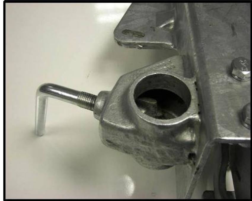
**The locking handle is wound into the jockey bracket and the pressure pad slots over the end of the handle. The handle then withdraws the pad securely into the housing casting where it is retained, making it impossible for either the pad or the handle to be lost. The handle is M16 so extremely robust.**
