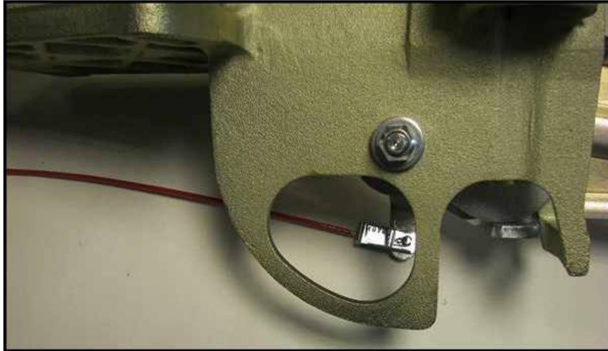
**Another longstanding feature on all cast couplings since 1993, the skid is an integral feature of the cast housing and protects the overrun lever and handbrake lever from damage from sleeping policemen and other objects under the trailer. This feature is mandatory in many European countries.**
